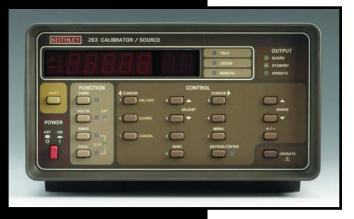
The Model 263 Calibrator/Source is a secondary standard for use when calibrating electrometers and picoammeters (or wherever precise low current, high resistance, voltage, or charge is needed). Designed for use as a multifunction calibrator/source, the Model 263 can source current, resistance, voltage, and charge. A built-in voltage source provides  $5\mu V$  to 20V. Where more than 20V is required, the Model 263 can switch up to 200V from an external voltage source to its output terminals.
